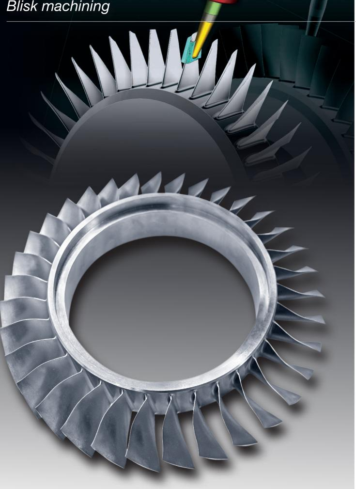
The turn-milling center featuring a horizontal part arrangement is especially suited for the machining of turbine and compressor blades, blisks or radial compressors. Here, the configuration of the working area ensures optimum mass distribution, as well as good visibility of the machining situation.
