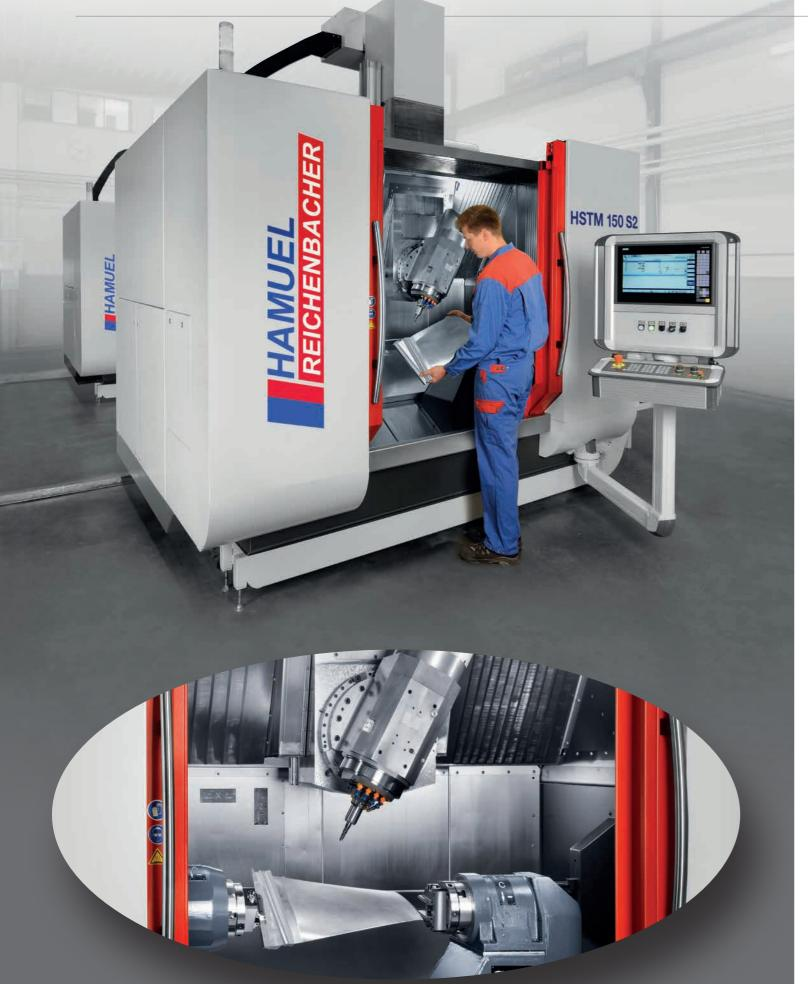
Mineral cast machine base for unequaled vibration absorption and rigidity paired with extreme acceleration
