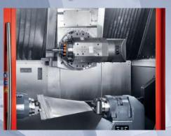
Extremely wide swivel range of the milling spindle
