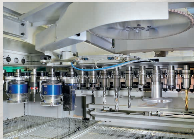
The automatic chain changer for 61 tools is mounted inside the portal enclosure behind the working unit.
