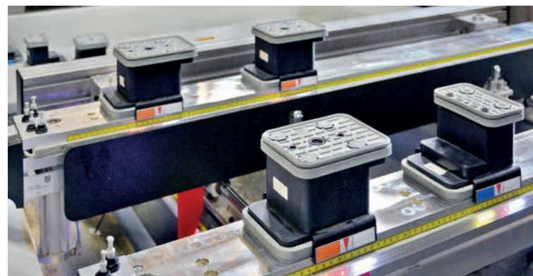
There are LED-positioning strips on the machine bed and on the individual beams to indicate the position of the beams and of the suction cups.
