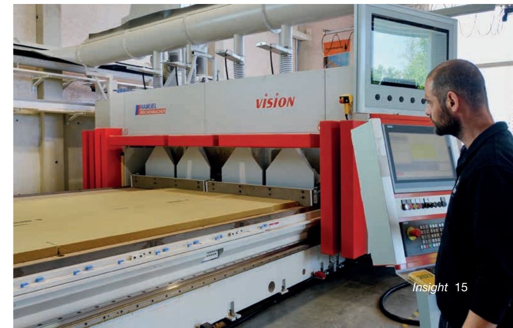
Lip channel extraction and push-off unit, which permit the processing of panels up to 14 metres in length.
