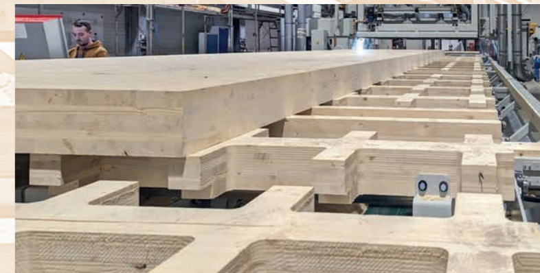
Equipped with a steel beam table with wooden supports and conveyor technology, very large CLT panels can be processed.
