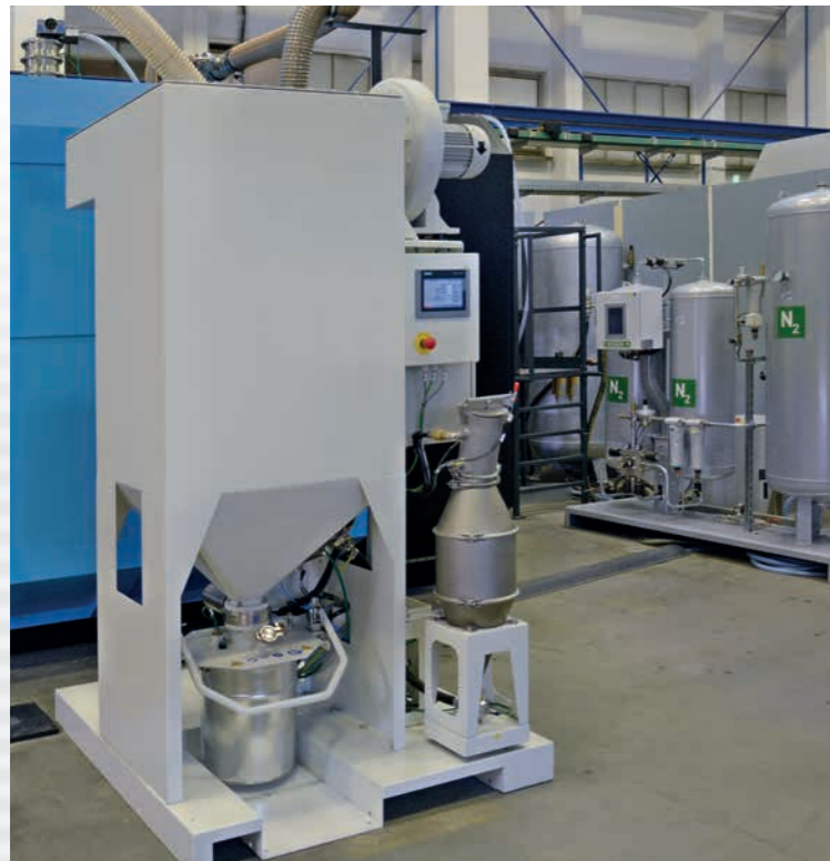
Extraction system Fume extraction system (filtration) with a sinter-plate filter in combination with safe passivation and integration into the inert gas circulation system.
