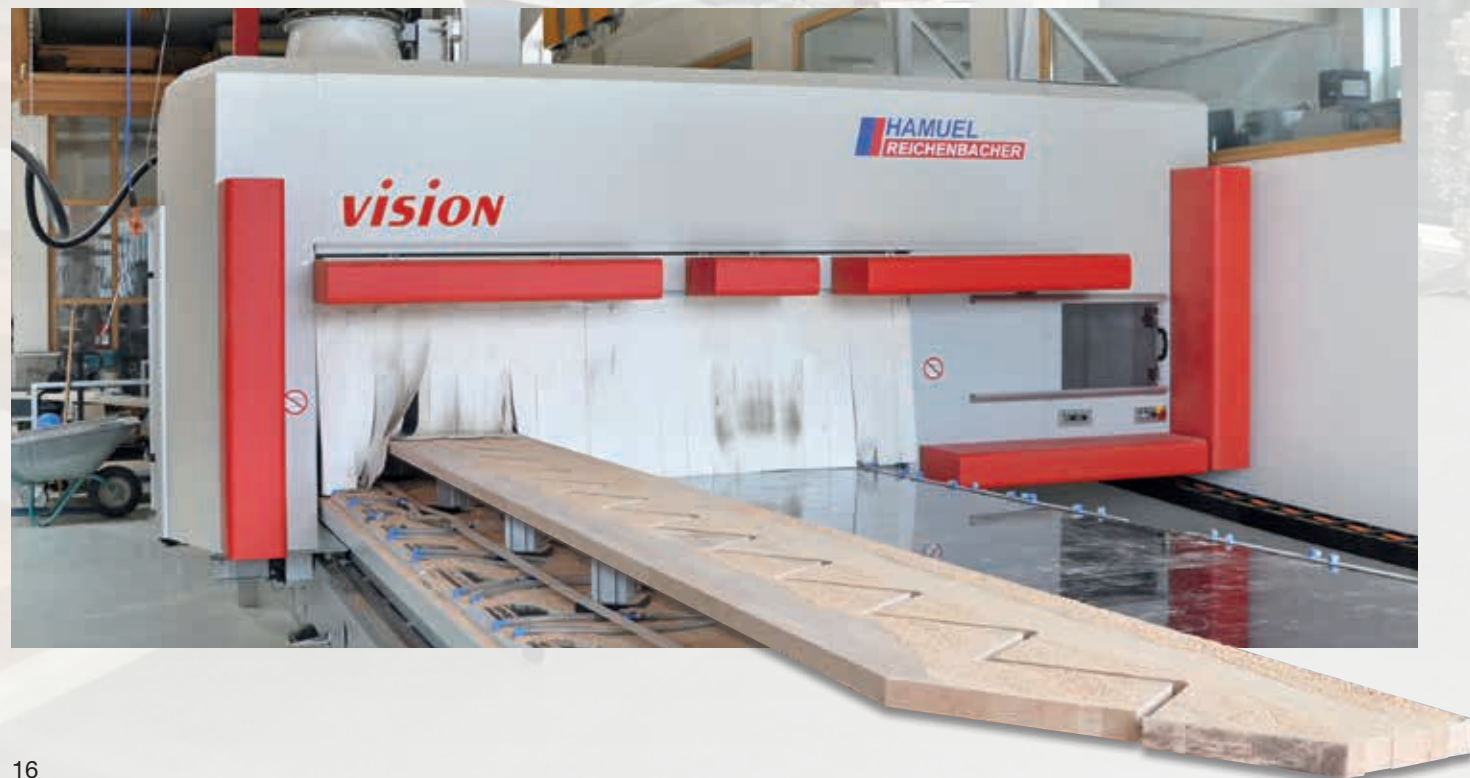
Picture below: CNC-machining centre VISION-II-T with multifunctional grooved table to be used for nesting, plane surface for double-acting suction cups.
