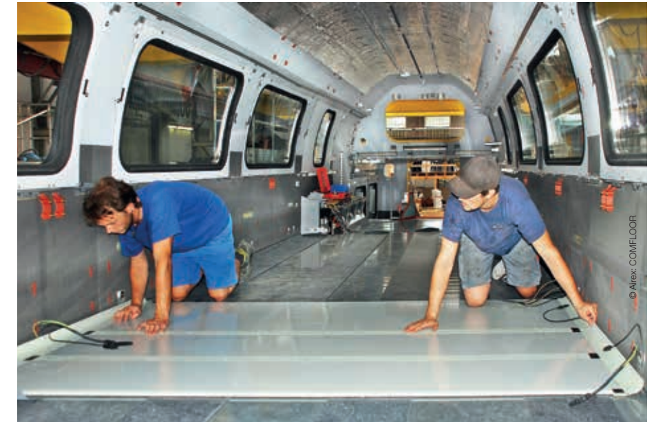
Top: Heatable floor systems (COMFLOOR®) for railway vehicles are developed and manufactured precisely to customer requirements.
