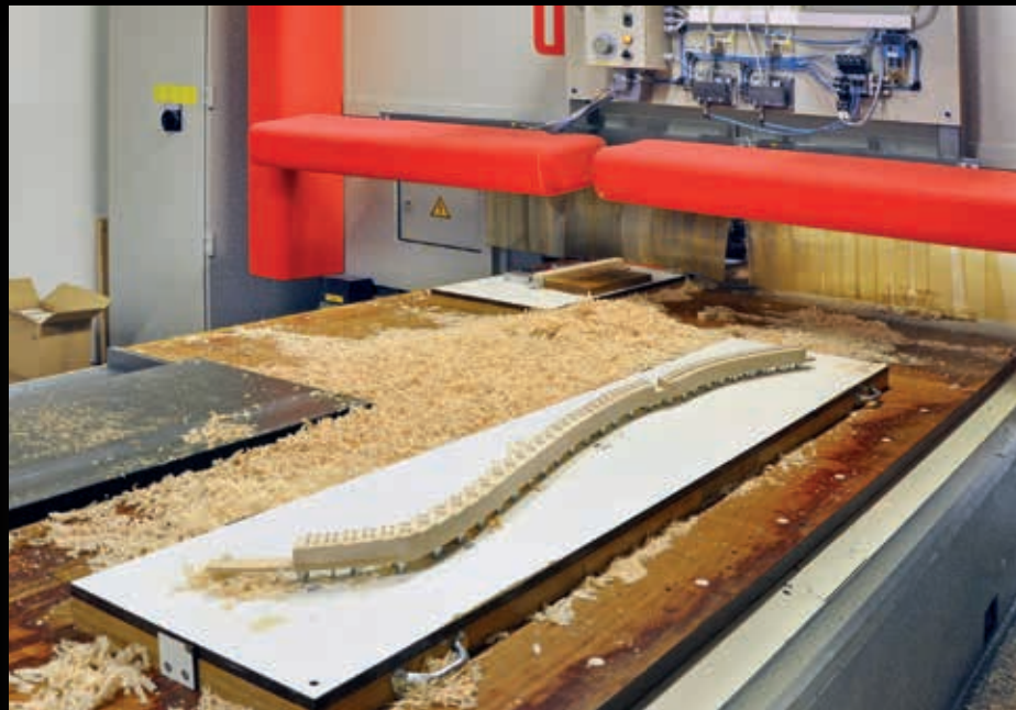
Finished long bridge of an upright piano (formatted, holes drilled, recesses milled and pins inserted) on a Reichenbacher UNIVERS.
