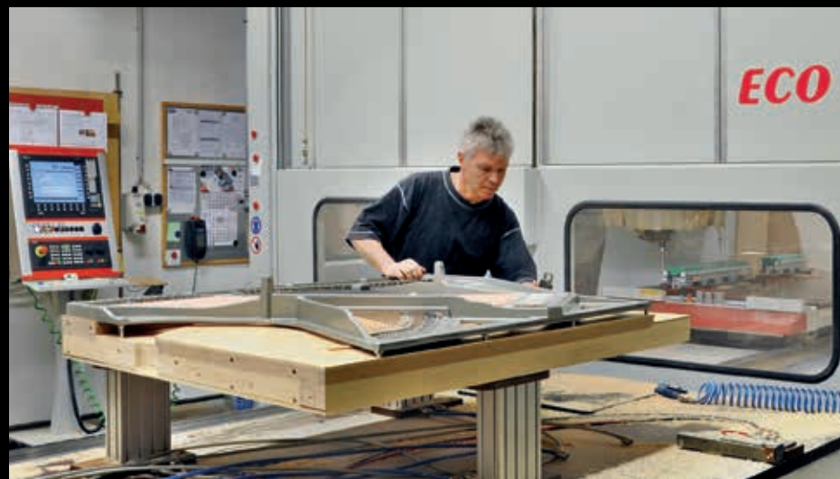
Picture left: Acoustic assembly of an upright piano completely formatted on a Reichenbacher ECO-1625-B Sprint.
