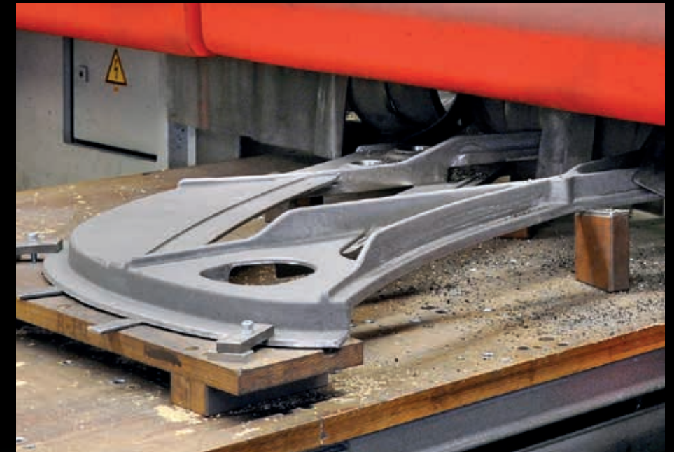
Cast-iron frame for a grand piano on a Reichenbacher VISION.
