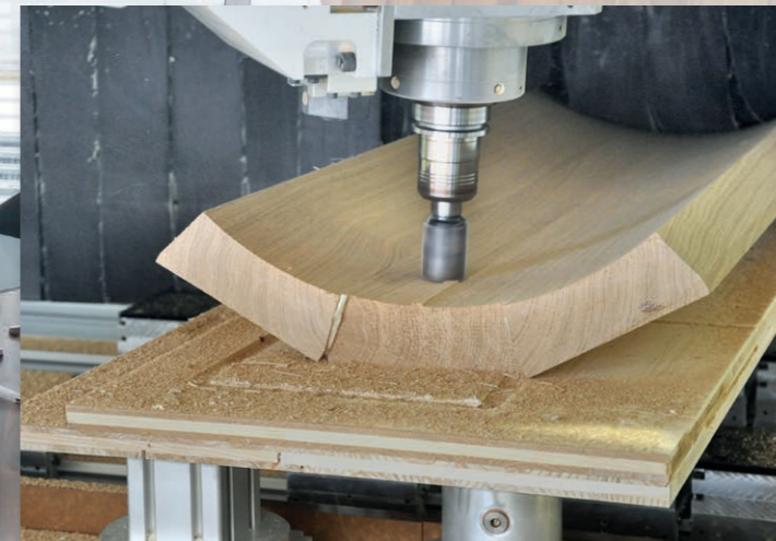
5-axes machining of a round newel post.
