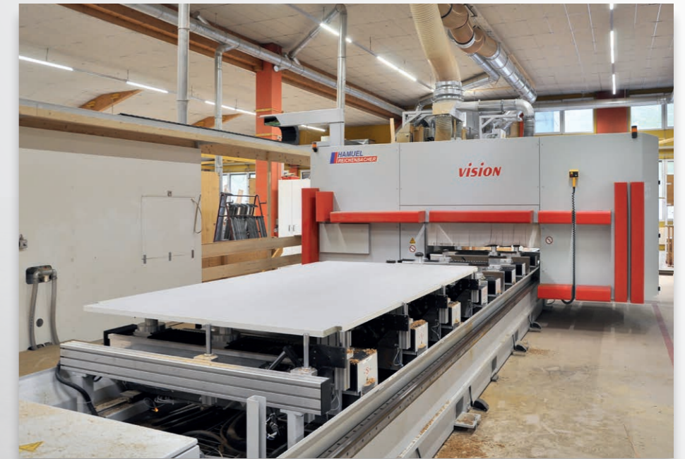
CNC-machining centre VISION-II Sprint in stop position after machining with component still in place.
