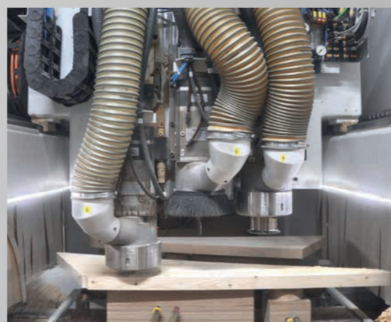
At Sonnemans the VISION-II-ST Sprint is equipped with a 5-axes head and with three additional units.
