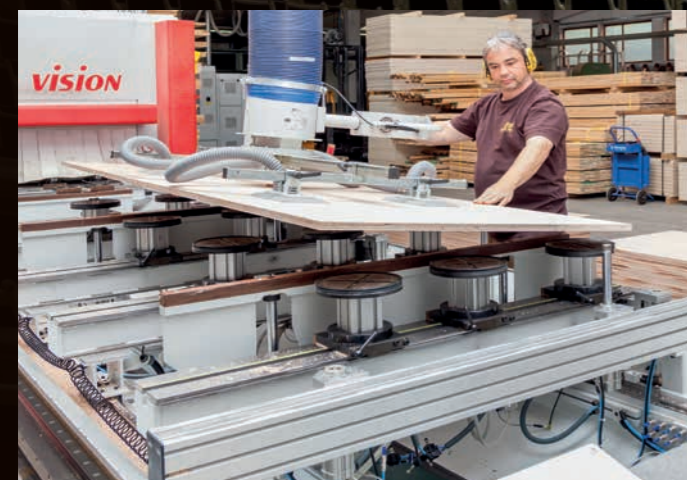
The CNC-machining centre and the vacuum tube lifter from J. Schmalz form a perfect duo.
