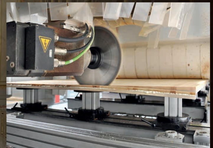
Heavy materials are used in stage building. A robust machine bed is absolutely necessary for the machining of the plates weighing 180 kg.
