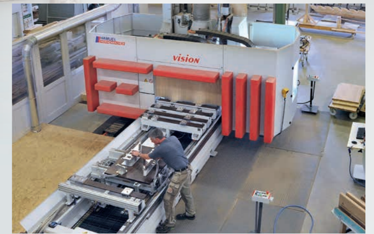
Machining centre with 5-axes unit and 3x vertical spindles, which has specifically been designed for staircase manufacturing, in the Meyer & Grave factory.
