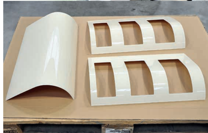
◀ The panel for the spice rack before and after machining.
