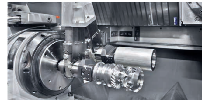
Changer with double gripper: Constant availability of tools and workpieces.
