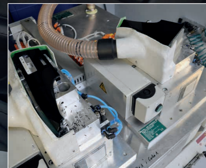
The devices are carried out for the simultaneous machining of two components per plate.
