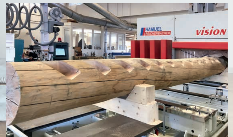
Machining of the log on the CNC-machining centre VISION-ST-H took eight hours.
