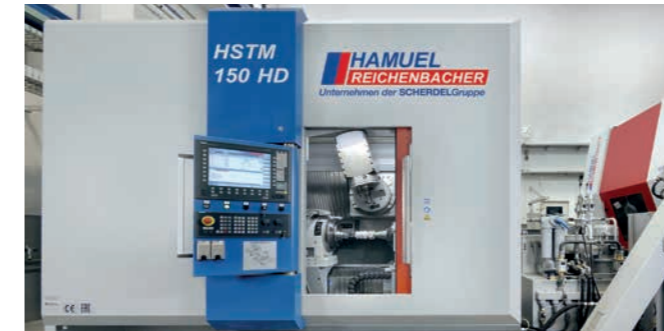
HSTM 150 HD: CNC-milling solutions for 5-axes machining.
