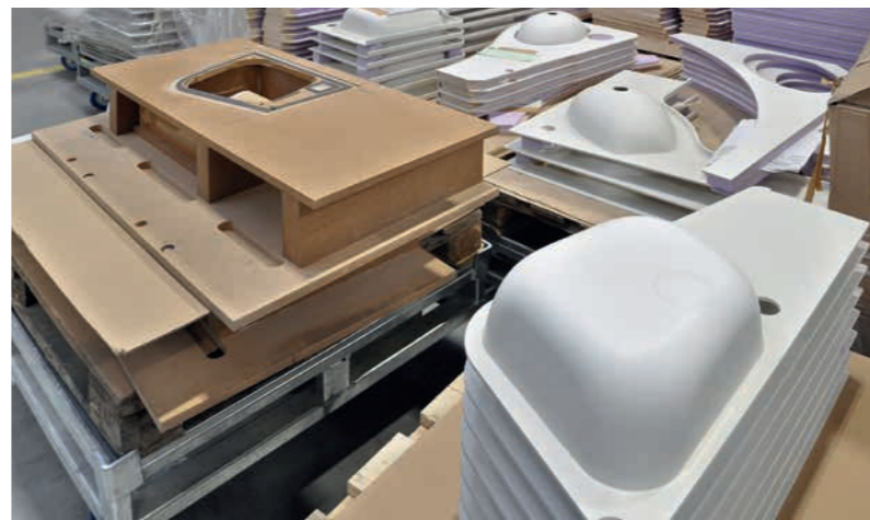
▼ Various washbasins after machining.
