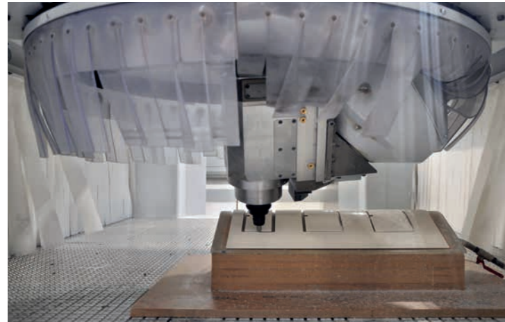
▲ Machining of the outer panel of a spice rack from acrylic glass.
