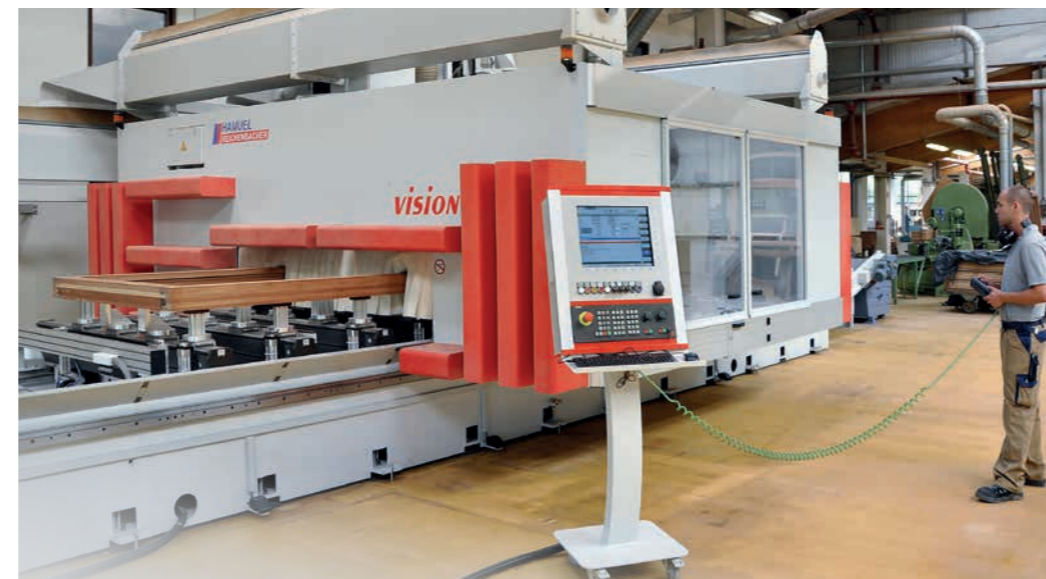
The Reichenbacher engineers have specifically customised the 5-axes machining centre VISION-III-T-U for Hoba's particular requirements.
