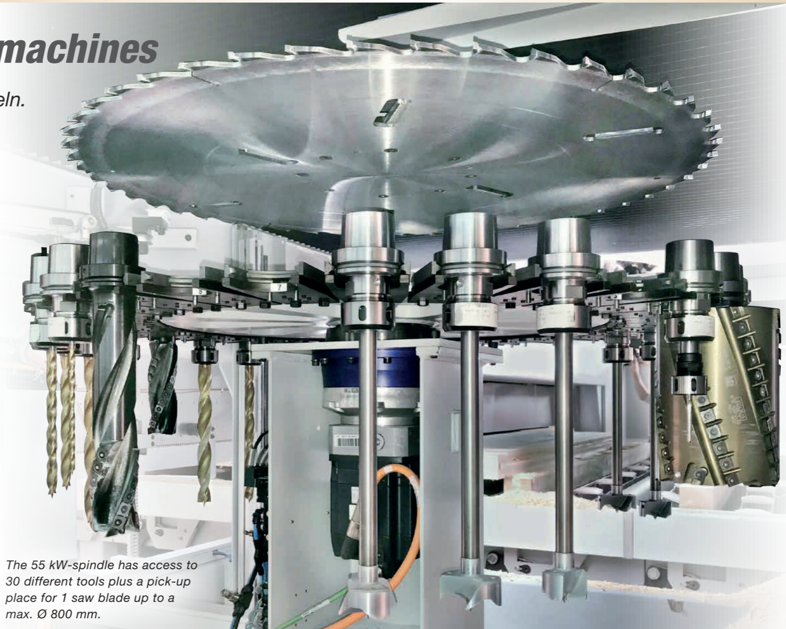
Derix at Westerkappeln are working with very compact and powerful 5-axes CNC-machining centres.
