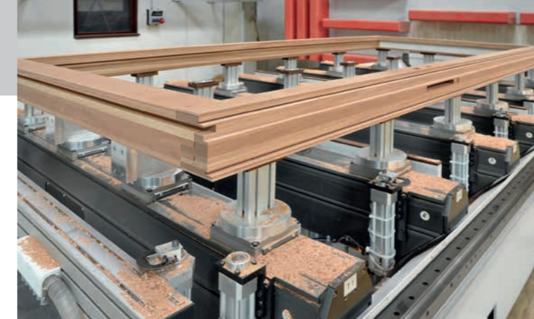
The fully automated beam table is comprehensively equipped for all the complete machining operations that can be imagined. Even clamps for the posts have been included.
