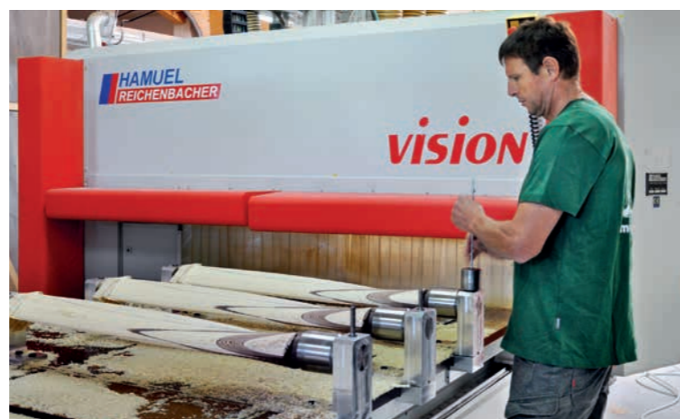
Alois Kermer at a CNC-machining centre type VISION Inline. The propeller blades are turned around in special fixtures to permit the milling of the blade's bottom side.
