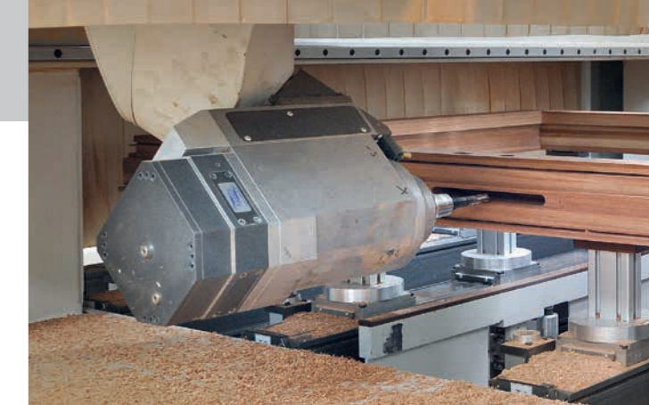
The 5-axes unit is ideally suited e.g. for the horizontal millings for locks, as it saves an extra unit for lock cases.
