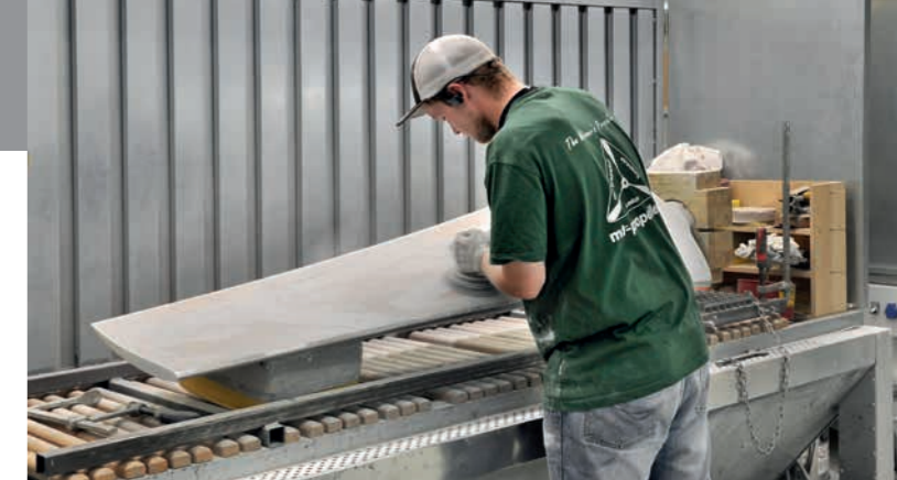
Grinding of the propeller blade subsequent to the application/drying of the primer. This must be done manually.
