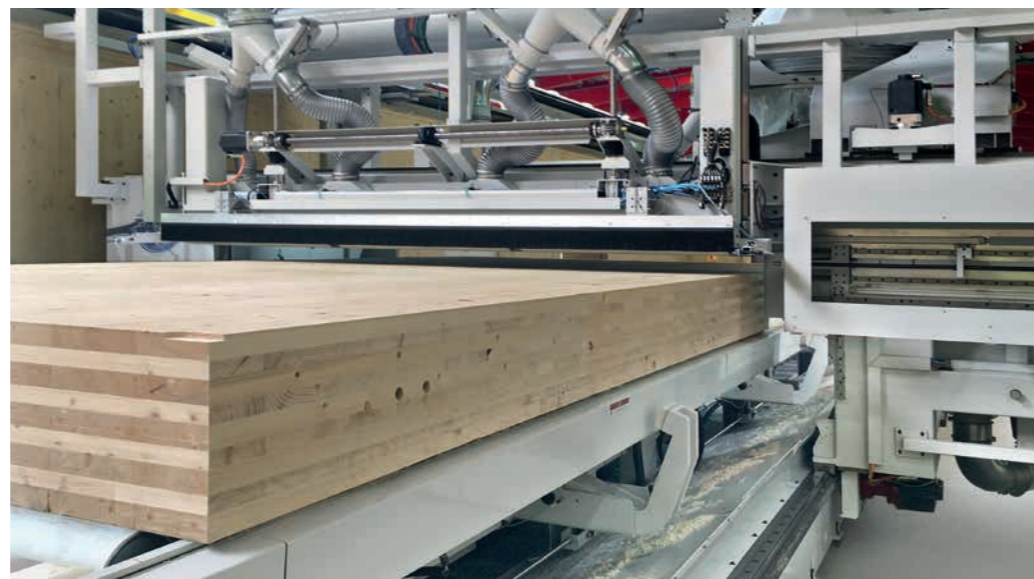
Component transport inside the machine is ensured by a roller track and a cross conveyor.
