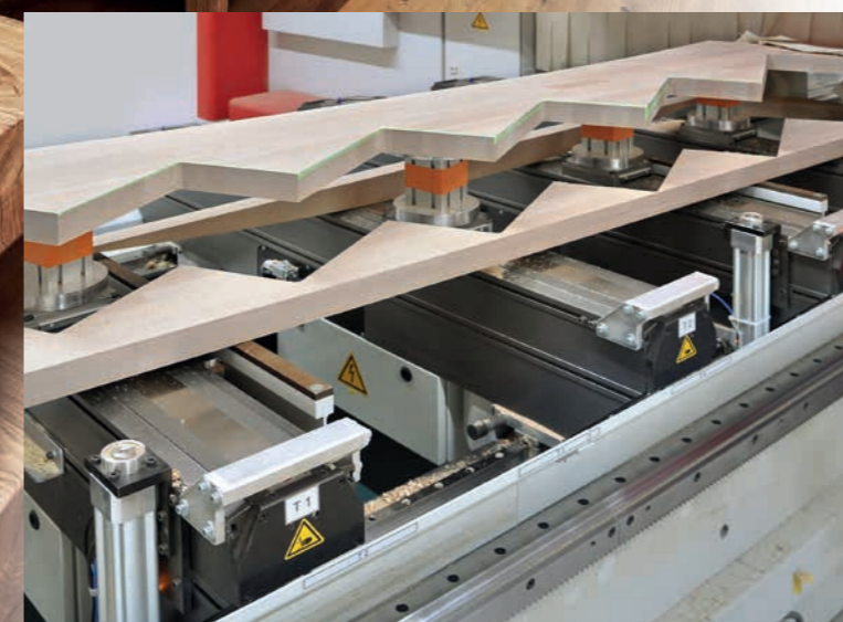
Now, strings of up to 6.50 m in length including face machining can be manufactured.
