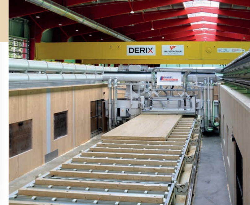
Derix at Westerkappeln are working with very compact and powerful 5-axes CNC-machining centres.
