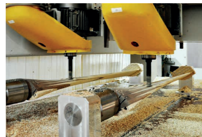
Rough milling is followed by fine milling operations, which take about 25 minutes per side for a small propeller blade.
