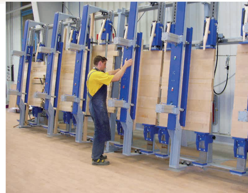
Workmanship with tradition: many production steps at Dietel are manual ones – gluing, too.
