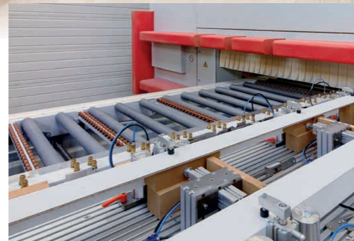
The CNC-machining centre is a through-feed line equipped with roller tracks.
