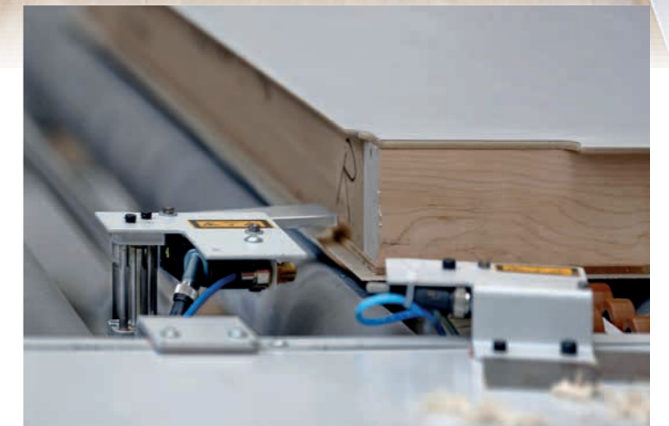
Linear stop for pneumatic positioning intended for a maximum veneer overhang of 1 - 50 mm.
