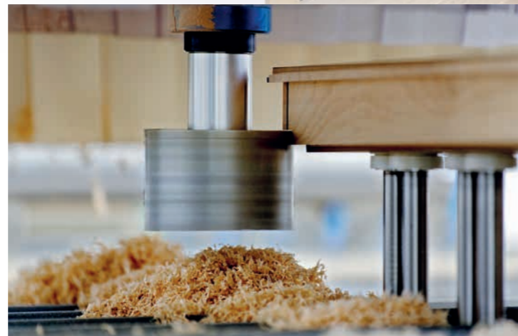
Door machining: flexibility for doors with special rebates, milling in all planes due to the free accessibility of the doors.
