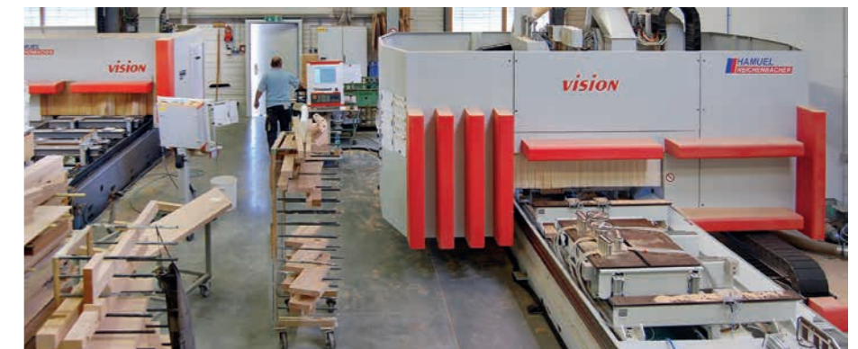
The VISION-II-ST 5-axes permits the processing of components up to a total length of 6,900 mm.
