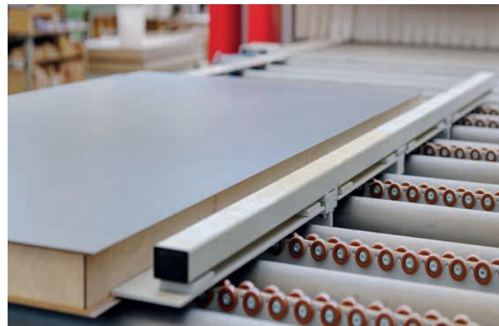
Aligning equipment with pneumatic lifting on multiple roller strips intended for the alignment of the components in the Y-direction.
