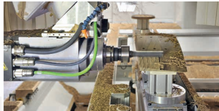
Machining of a round chair back.
