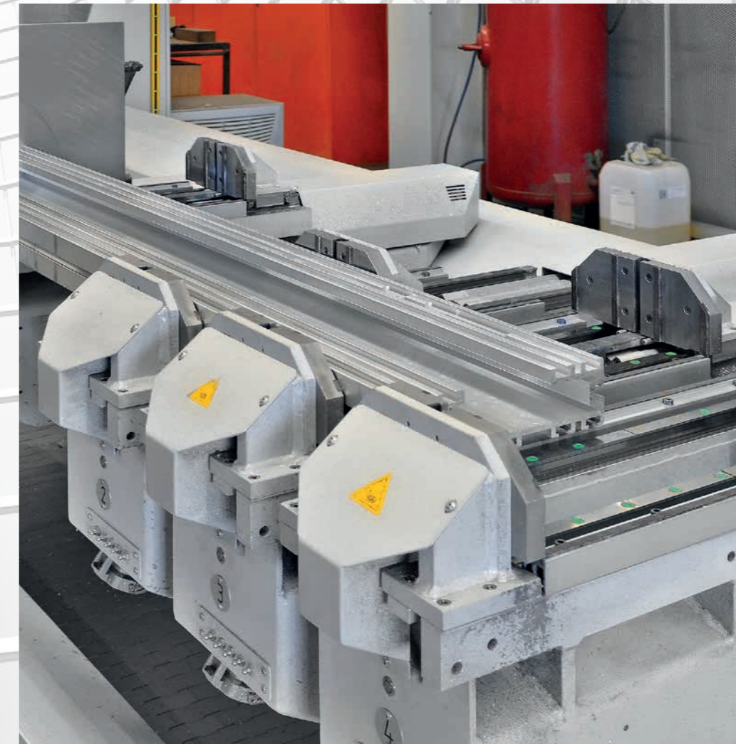
Clamping jaws or hold-downs precisely matched to the components are important for highly accurate milling results.
