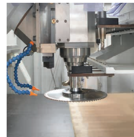
The synchronous motor allows fast sawing with saw blade diameters up to 450 mm.
