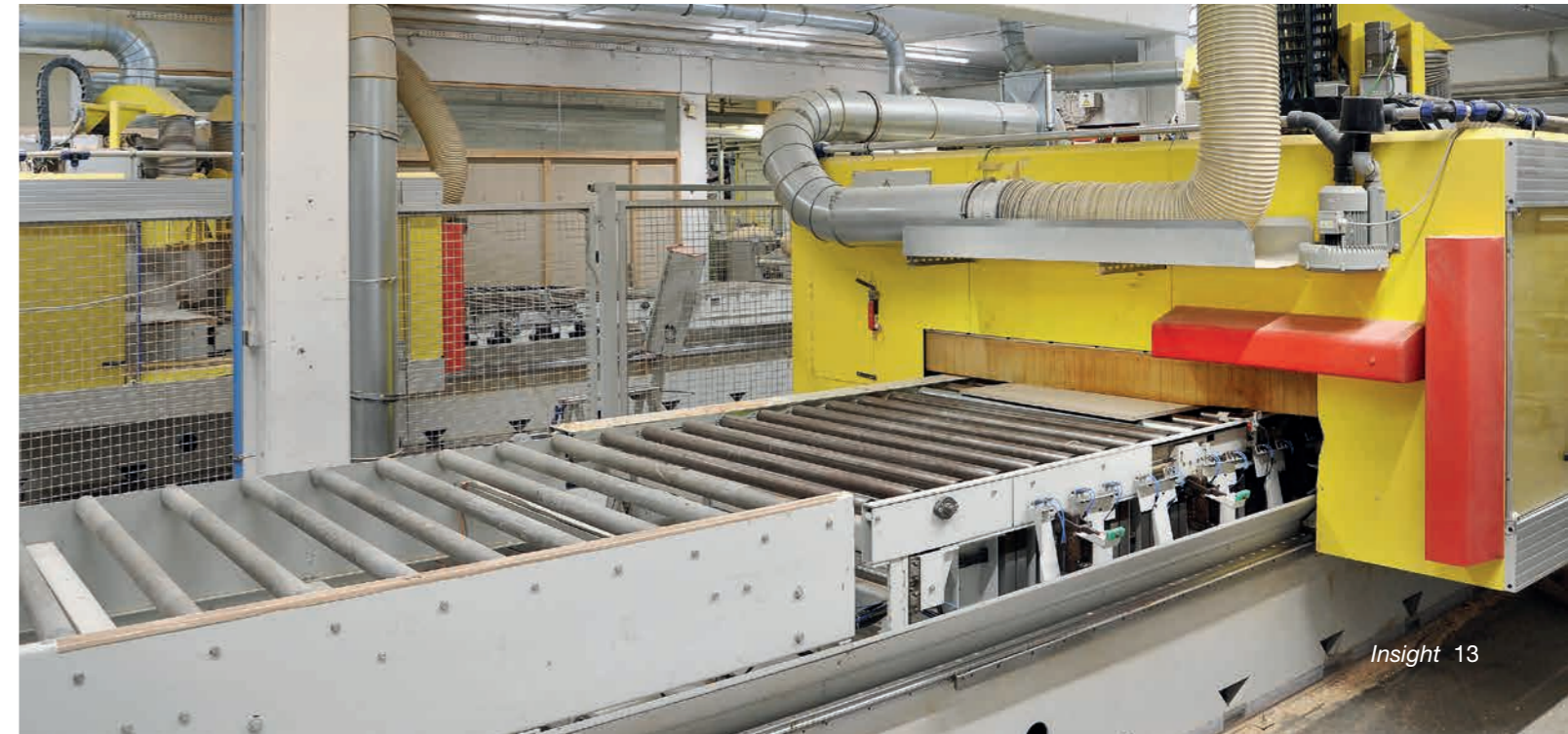
The through-feed table is equipped with a driven roller track with lifting device.
